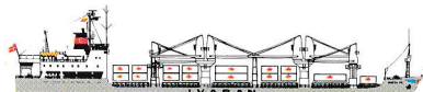
"SANTA FE" — Semi-containervessel, built 1978. 14.770 dwt/447 TEUs + 2 coiled/coated deep tanks for liquid cargo, of 11.410 cbft each. Speed: about 16,5 knots. Accommodation for 12 passengers.
