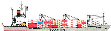
"SAVANNAH" — Semi-containervessel, built 1984. 12.540 dwt/700 TEUs + 2 coiled/coated deep tanks for liquid cargo, of 11.300 cbft each. Speed: about 17 knots.
