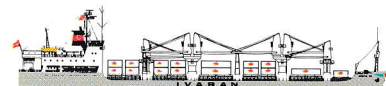
"SALVADOR" — Semi-containervessel, built 1978. 14.770 dwt/447 TEUs + 2 coiled/coated deep tanks for liquid cargo, of 11.410 cbft each. Speed: about 16,5 knots. Accommodation for 12 passengers.
