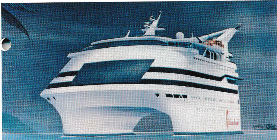
SCC Radisson Diamond – 18,400 ton – 410 ft. long – 105 ft. wide with a draft of 23 – 26 feet.
