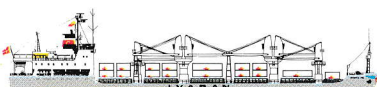
"SANTA FE" — Semi-containervessel, built 1978. 14.770 dwt/447 TEUs + 2 coiled/coated deep tanks for liquid cargo, of 11.410 cbft each. Speed: about 16,5 knots. Accommodation for 12 passengers.
