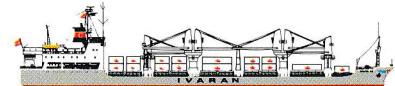
"SALVADOR" — Semi-containervessel, built 1978. 14.770 dwt/447 TEUs + 2 coiled/coated deep tanks for liquid cargo, of 11.410 cbft each. Speed: about 16,5 knots. Accomodation for 12 passengers.
