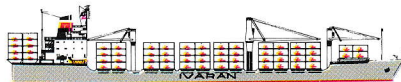
"SAVANNAH" — semi-containervessel, built 1984. 13.800 dwt/958 TEUs + 2 coiled/coated deep tanks for liquid cargo, of 11.300 cbft each. Speed: abt 17 knots.
