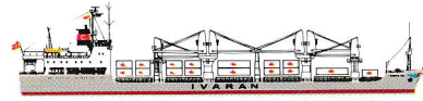
"SANTA FE" — Semi-containervessel, built 1978. 14.770 dwt/447 TEUs + 2 coiled/coated deep tanks for liquid cargo, of 11.410 cbft each. Speed: about 16,5 knots. Accomodation for 12 passengers.
