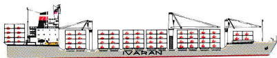
"SAVANNAH" — Semi-containervessel, built 1984. 13.800 dwt/958 TENS + 2 coiled/coated deep tanks for liquid cargo, of 11.300 cbft each. Speed: abt 17 knots.
