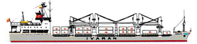
"SANTA FE" - Semi-containervessel, built 1978. 14.770 dwt/447 TEUs + 2 coiled/coated deep tanks for liquid cargo, of 11.410 cbft each. Speed: about 16,5 knots. Accomodation for 12 passengers.
