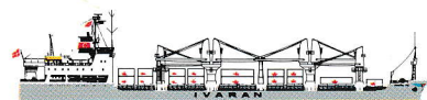
"SALVADOR" - Semi-containervessel, built 1978. 14.770 dwt/447 TEUs + 2 coiled/coated deep tanks for liquid cargo, of 11.410 cbft each. Speed: about 16,5 knots. Accomodation for 12 passengers.
