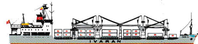
"SANTA FE" - Semi-containervessel, built 1978. 14.770 dwt/447 TEUs + 2 coiled/coated deep tanks for liquid cargo, of 11.410 cbft each. Speed: about 16,5 knots. Accommodation for 12 passengers.
