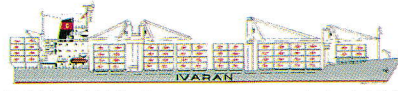
"SAVANNAH" - Semi-containervessel, built 1984. 13.800 dwt/958 TEUs + 2 coiled/coated deep tanks for liquid cargo, of 11.300 cbft each. Speed: about 17 knots.
