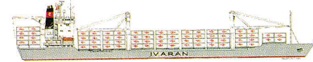
"SAN ISIDRO" - Containervessel, delivery December 1993. About 20.000 dwt/1512 TEUs (cellular). Speed: about 20 knots.
