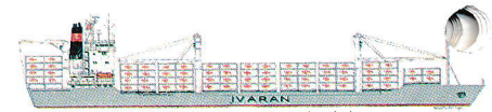
"SAN ISIDRO" - Containervessel, delivery December 1993. About 20.000 dwt/1512 TEUs (cellular). Speed: about 20 knots.
