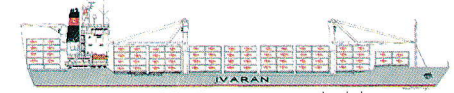
"SAN ANTONIO" - Containervessel, delivery March 1994. About 20.000 dwt/1512 TEUs (cellular). Speed: about 20 knots.
