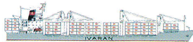
"SAVANNAH" - Semi-containervessel, built 1984. 13.800 dwt/958 TEUs + 2 coiled/coated deeptrunks for liquid cargo, of 11.300 cbft each. Speed: about 17 knots.
