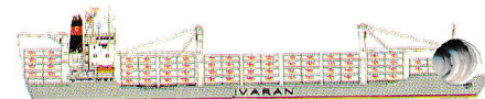
"SAN CLEMENTE" - Containervessel, delivery December 1994. About 20,000 dwt/1,512 TEUs (cellular). Speed: about 20 knots.
