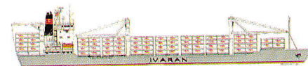
"SAN CRISTOBAL" - Containervessel, delivery December 1995. About 20,000 dwt/1,512 TEUs (cellular). Speed: about 20 knots.
