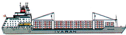
"AMERICANA" - Container/passengervessel, built 1988. 19,818 dwt/1,120 TEUs (cellular) + 3 coiled/coated deep tanks for liquid cargo of 11,785 cbft each. Speed: about 19 knots. Accommodation for 80 passengers.
