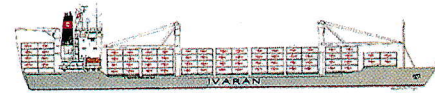
SAN FRANCISCO - Containervessel, delivery April 1996. About 20,000 dwt/1,512 TEUs (cellular). Speed: about 20 knots.
