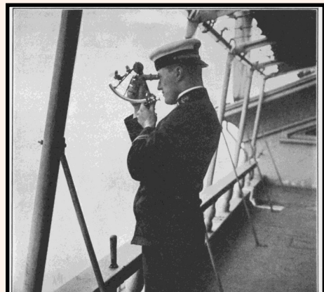
Brown Brothers The ship's officer finds the sun's altitude with a sextant
